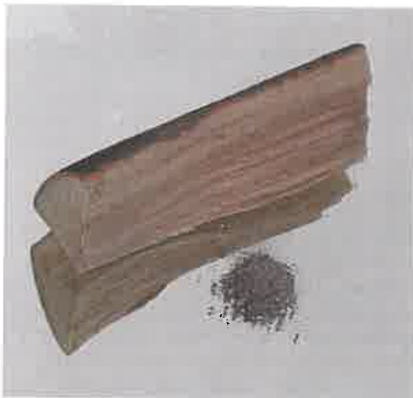
Picture: Approx. 5 grams of mineral ash remain after the burn of approx. 500 grams air-dry beech (20% moisture)
